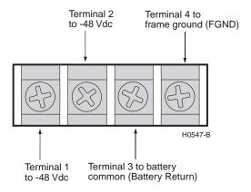
Figure 7. Connect -48 Vdc and Frame Grounds to TB1
